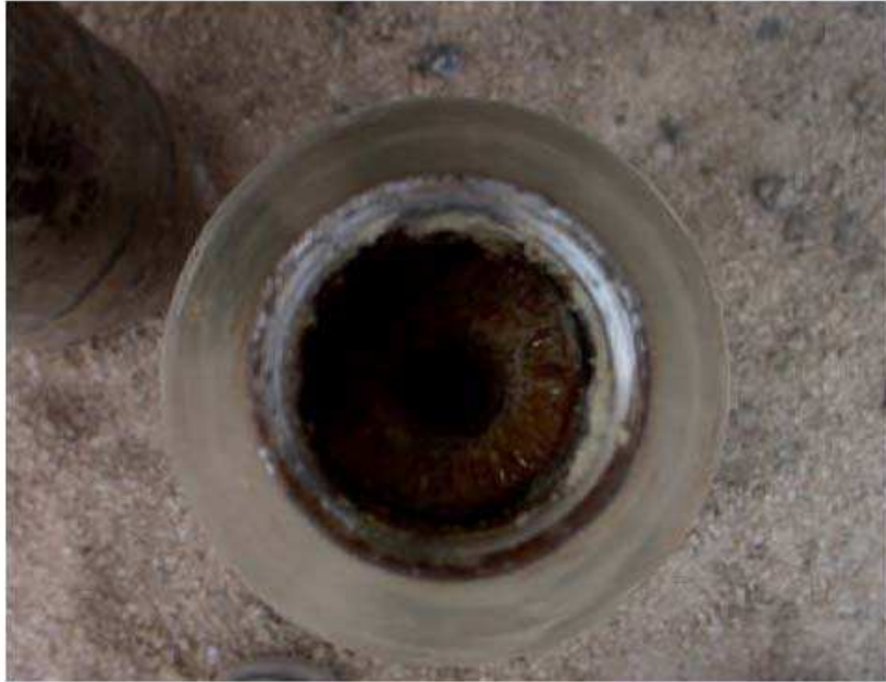
Top view of former Soviet Union 122mm Projectiles modified to accept a blasting cap in the cast high explosive (HE)
