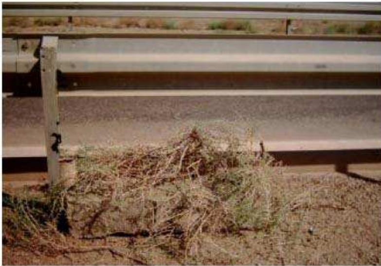
Projectile embedded in plaster of paris (POP) housing to simulate concrete covered with grass
