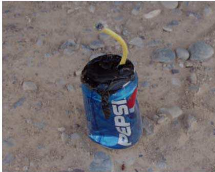
Modified Pepsi cola aluminum can with pyrotechnic fuse
