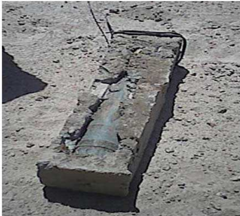
Projectile embedded in plaster of paris (POP) housing to simulate concrete
