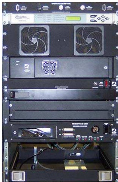
Figure 1-2 Rack Adapter Kit for AN/TSC-85D Terminal NSN: 5975-01-529-3943
