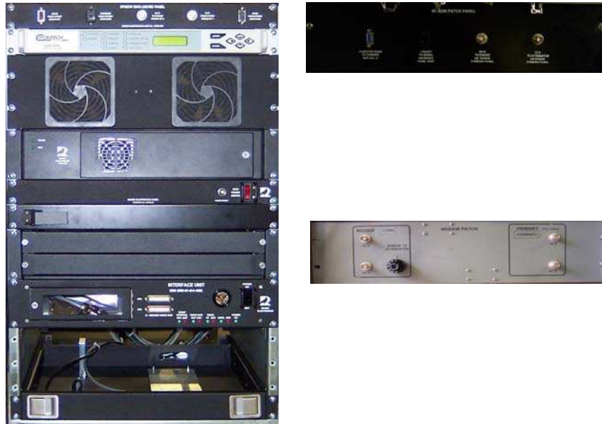
Figure 1-1 RFMOW for AN/TSC-85D Terminal NSN: 5895-01-522-2119
