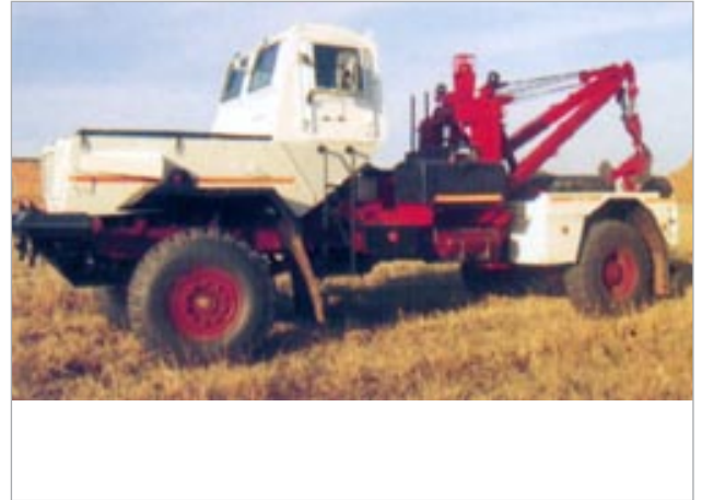
Samil 50 4x4 8 tons of Payload Armoured Cab & engine bay
