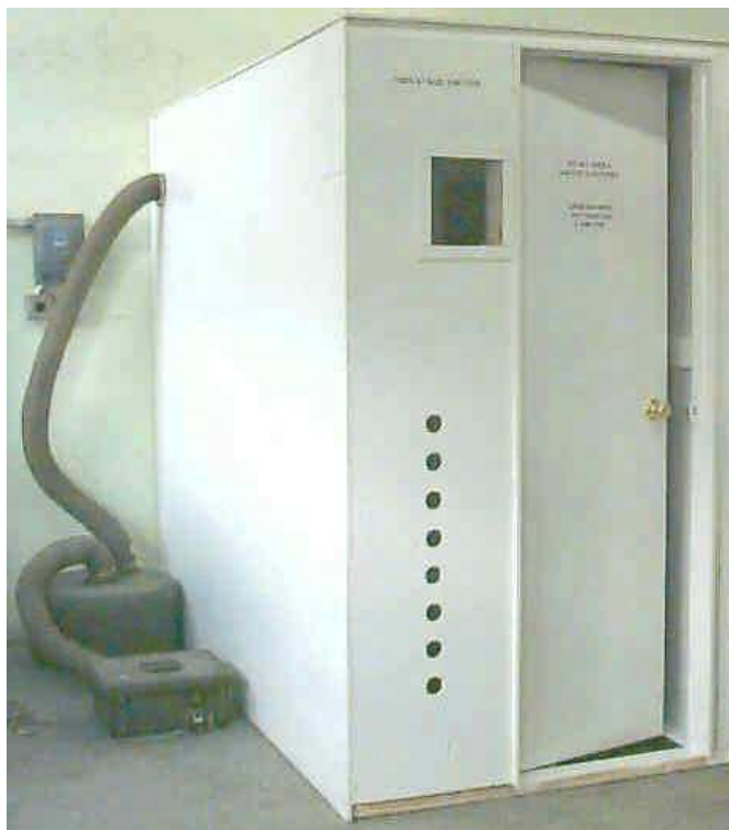
Figure J-5. Fabricated Airlock with Filter-Blower Unit
