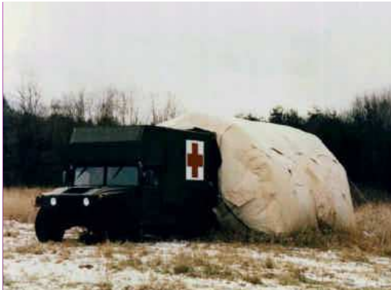
Figure J-10. Chemical Biological Protective Shelter (CBPS)
