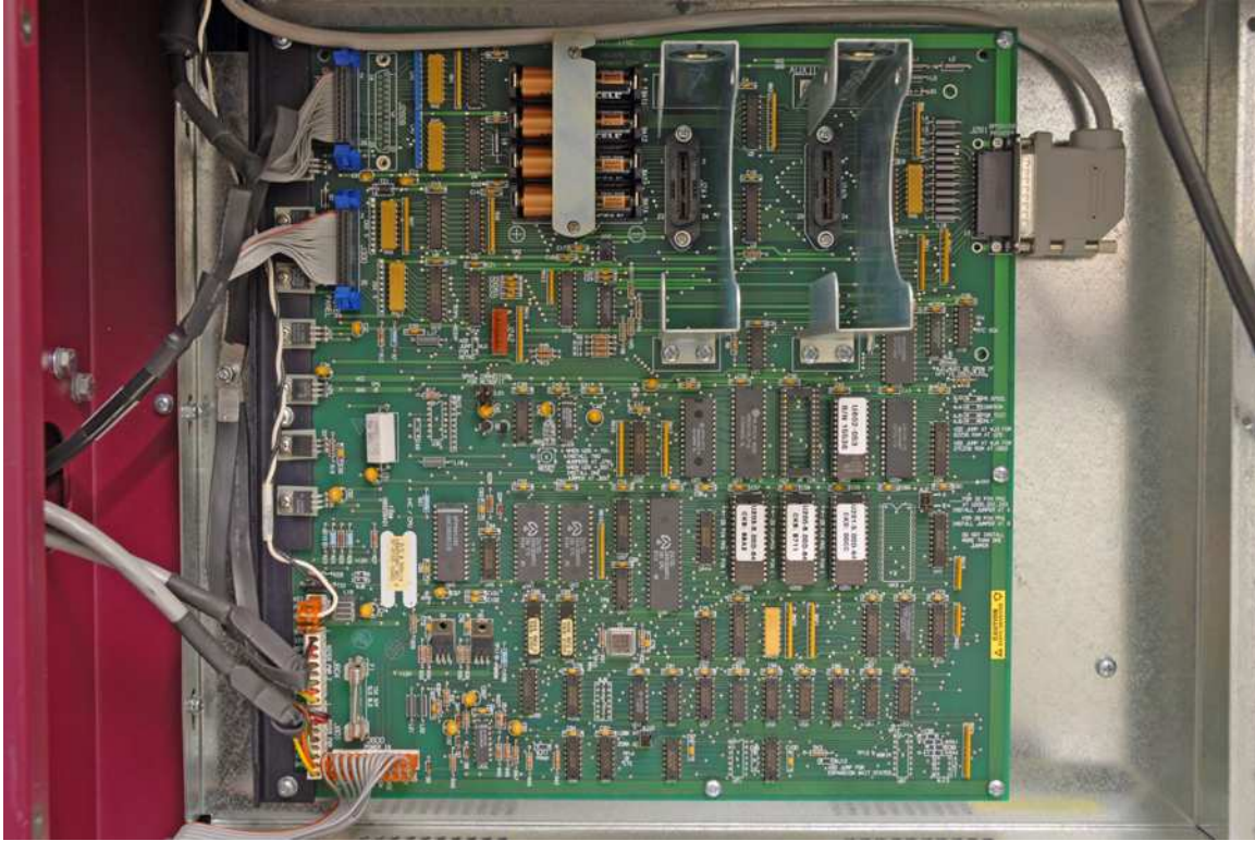
Figure 6: The motherboard of the AVC Advantage The Z80 is the largest chip, at center right. The ROMs have white labels. This machine is one that Appel purchased in 2007; the motherboards of the machines we examined from Union County, NJ are similar.
