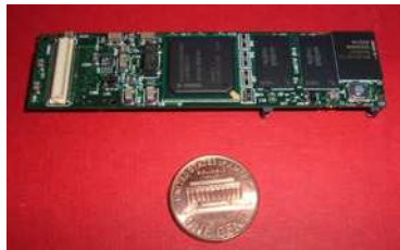
Figure 27: Tiny computer, sold for $99 by gumstix.com, that could be the “brains” of a cigarette-pack size device to alter the contents of Results Cartridges
