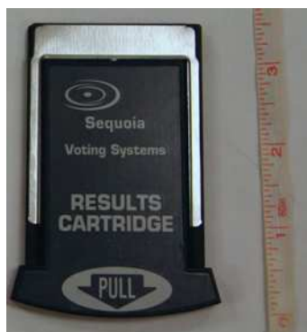
Figure 37: This cartridge, used only for audio ballots on AVC Advantage 9.00, is used as a Results Cartridge on AVC Advantage 10.
