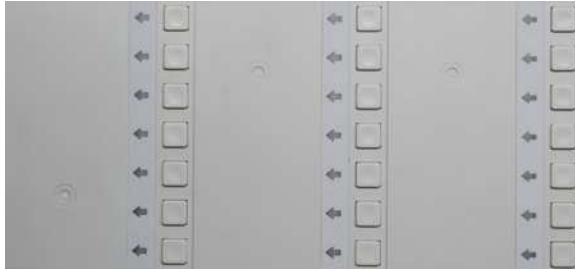
Figure 21: A small portion of the voter panel, without the printed paper ballot overlay.
