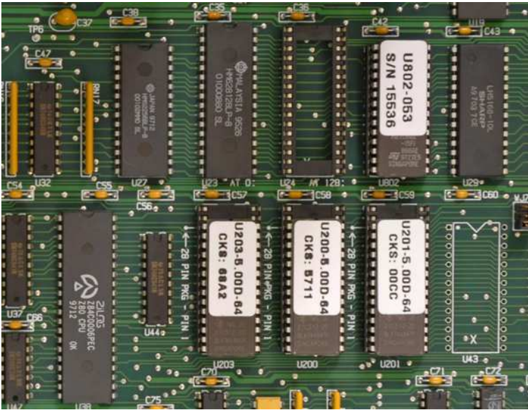
Figure 7: Z80 and ROM chips on the motherboard. The Z80 is the large chip at lower left. The ROMs have white labels.
