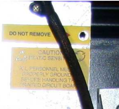
Figure 14: Close-up from Figure 5. The hole labeled DO NOT REMOVE contains no seal.
