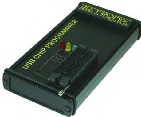
Figure 8: ROM reader/programmer; cost $150; approx. 3 inches by 2 inches
