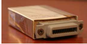
Figure 28: Nonfunctional mock-up of a device, in a cigarette pack, to alter the contents of Results Cartridges.
