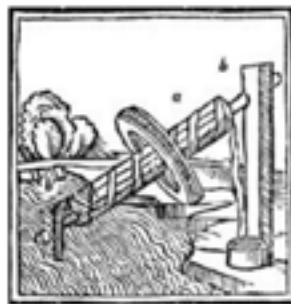
Archimedean Screw by Fra Gioconda, from 1522 edition of Vitruvius's De Architectura.
