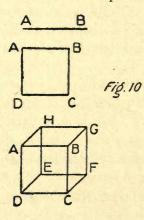
already familiar. The line AB, is bounded by the points A and B. (Fig. 10). The square, A B C D, is bounded by four lines AB, BC, CD, DA. The cube, A B C D E F G H, is bounded by six surfaces, namely, ABCD, CDEF, EFGH, GHAB, ADEH, BCFG.
