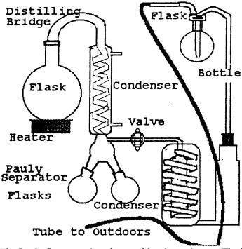
The Pauly Separator is to be considered mandatory. The lower condenser should be well insulated. The outer chamber is filled with cooling liquid. For example, 100 grams of ice with 143 grams of CaCl<sub>2</sub> -6H<sub>2</sub>O (Calcium chloride), will give a temperature of 55-60 degrees below 0 Celsius. This is easier to use than mixtures like acetone and dry ice.
