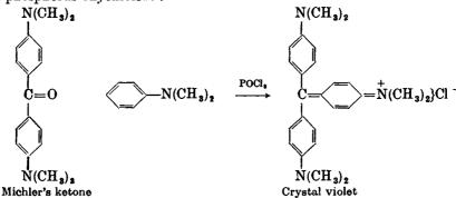
Michler's ketone is prepared industrially by the interaction of phosgene  $(COCl_2)$  and dimethylaniline.
