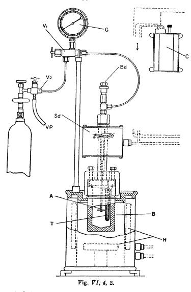
stainless steel, is the incorporation of a totally-enclosed agitator in the form of a plunger which is operated electro-magnetically; agitation efficiency is at least as high as is achieved with "shaking" autoclaves and is very effective for hydrogenation purposes. The apparatus is
