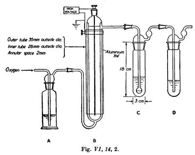
structed of soft soda-glass tubing (Pyrex glass is unsatisfactory): the glass should be thoroughly cleaned and the annular space through which the oxygen passes should be as uniform as possible. The complete apparatus should be placed in a fume cupboard (hood) behind a shatterproof screen of laminated safety glass.
