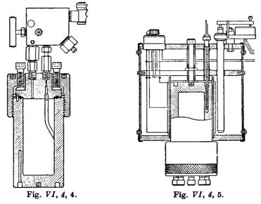
bomb head containing a rupturable disc which will burst at approximately 6,000 lb. per square inch. The temperature of the bomb and its contents is observed by means of a copper - constantan thermo-couple inserted in a copper cup in the bottom of the bomb. The electric heater is controlled by a variable - voltage transformer mounted on the base of the apparatus.
