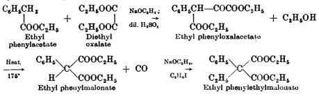
Ethyl phenylmalonate. In a l-litre flask, equipped with a dropping funnel, mercury-sealed stirrer and reflux condenser,\* place 11.5 g. of clean sodium picces (see Section III,7, Note 1); add 250 ml. of "superdry" ethyl alcohol (Section II,47,5) and allow the vigorous reaction to
