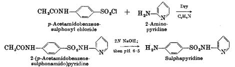
The 2-aminopyridine is prepared by adding pure, dry pyridine to sodamide in dry toluene at  $110^\circ$ :
