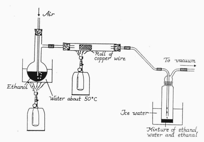
The partial oxidation of the alcohol takes place in the horizontal tube where the copper mesh acts as a catalyst for the reaction. The equation representing this is:
