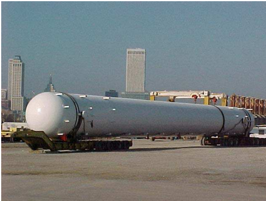
Figure 8-1. Large bulk chlorine storage tank manufactured by Trinity Industries with the flanged man-way located at the far right (bottom) of the tank.
