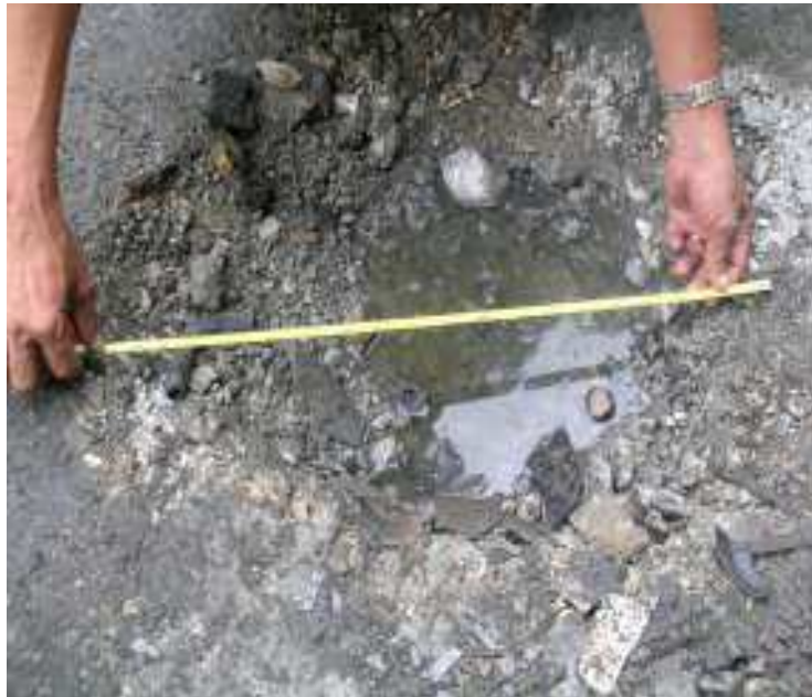
Figure 5: Seat of Explosion found underneath the vehicle measuring about 21"x 4" diameter deep crater
