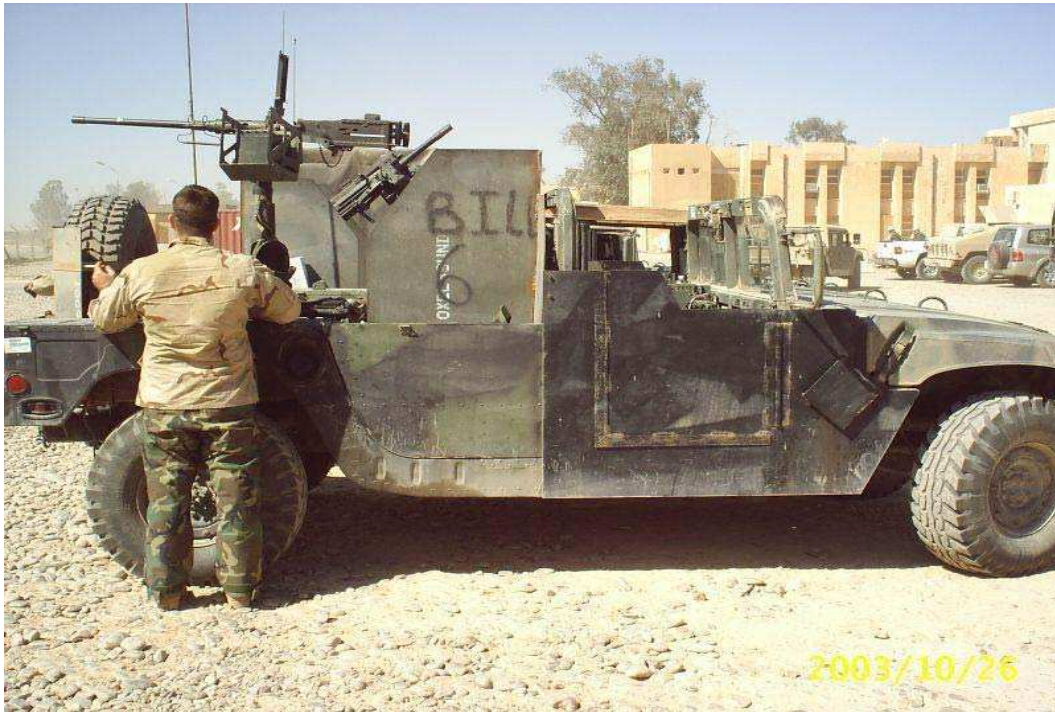
Figure 6-2. Vehicle Hardening and Pedestal Mount
