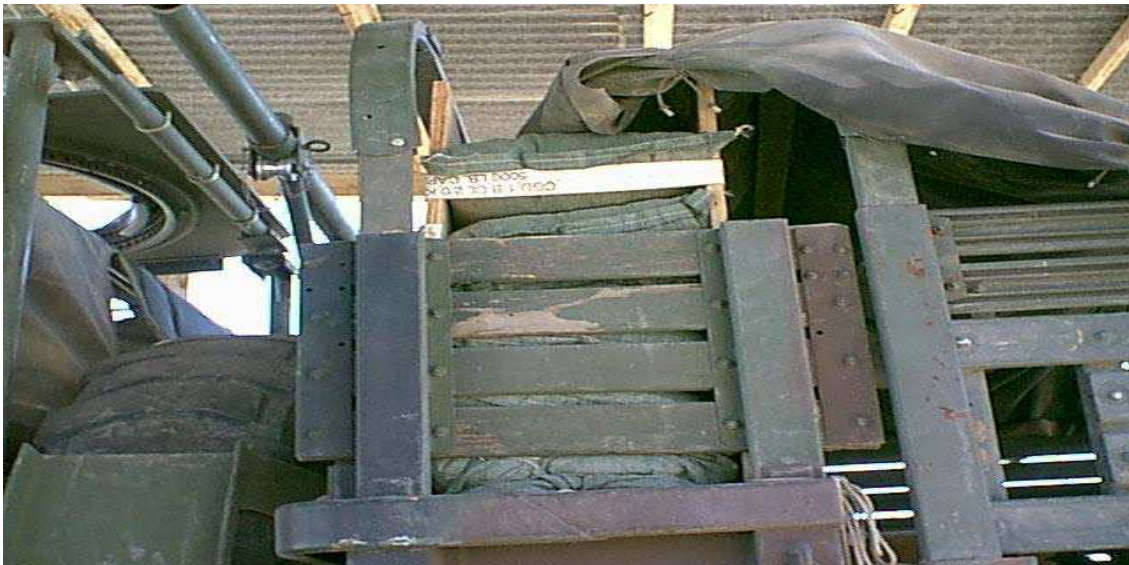
Figure 6-1. Vehicle Hardening (Notice Sandbags)
