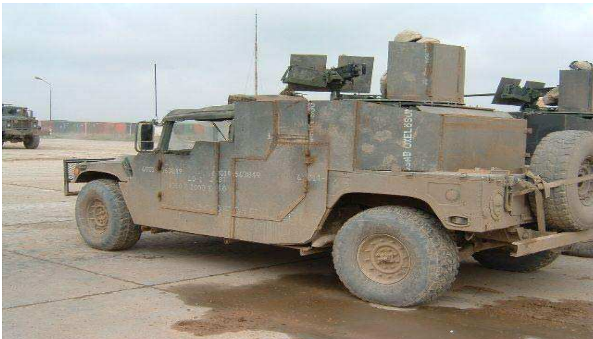
Figure 6-3. Gunner Shields to the Rear and Front
