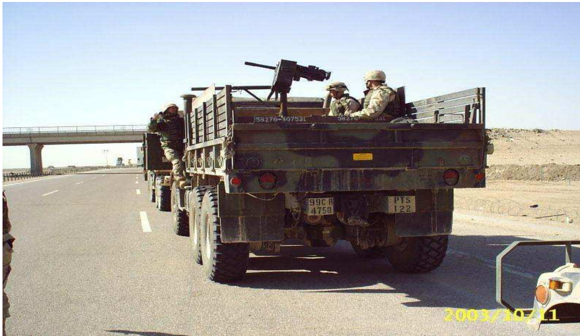
Figure 6-4. Armor Plating Surrounding the Gun Platform
