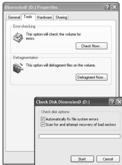
Figure 7-5: Use Check Disk to perform a complete surface scan.
