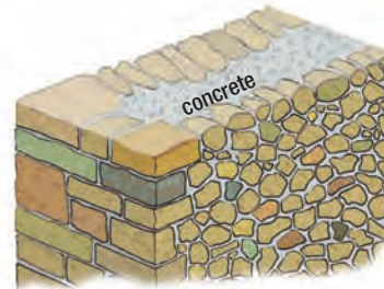
Right: Opus testaceum is a facing made of fired bricks cut into triangles; rectangular bricks are also used. An outer facing of thin travertine or marble panels covers many public buildings.
