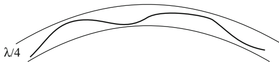
Fig. 7.20 The irregular shape of a wave surface cannot be distinguished from the perfect one if the differences are smaller than \lambda/4
