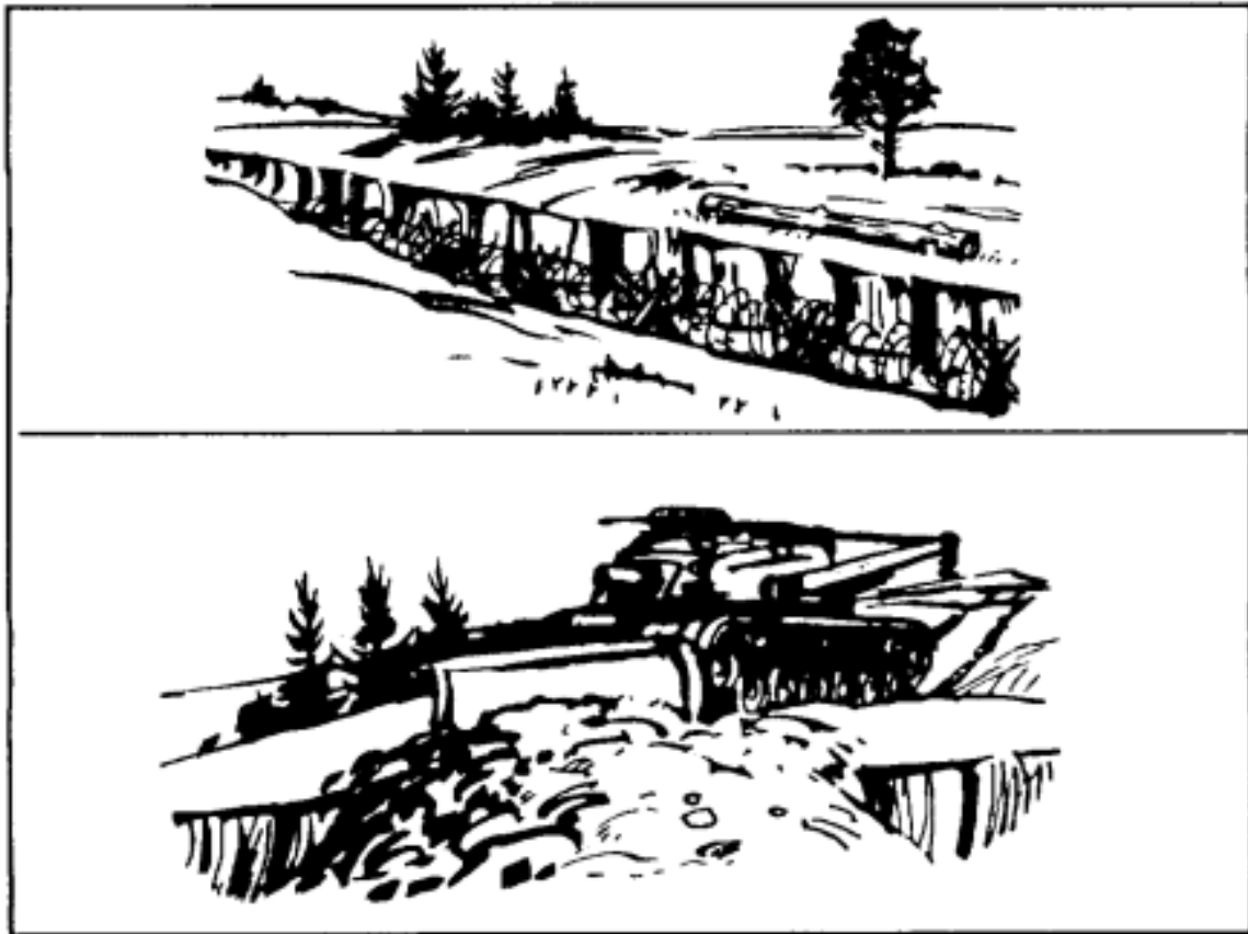
Figure 2-84. Clearing a tank ditch.
