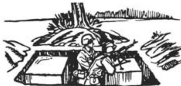
Figure 6-67. T-Shaped Position; Firing Primary Sector.
