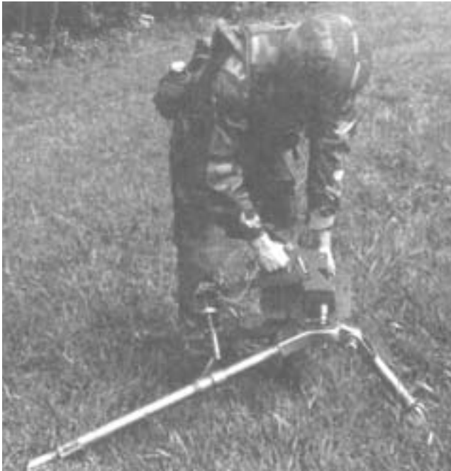
Figure 5-51. Mounting the Cradle on Tripod.
