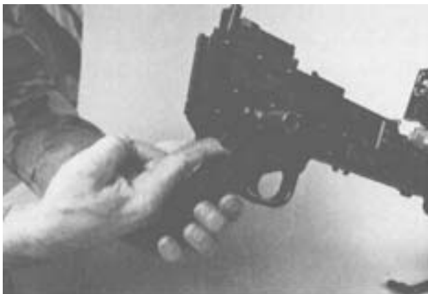
Step 1. Remove the Trigger Housing Assembly Spring Pin.
