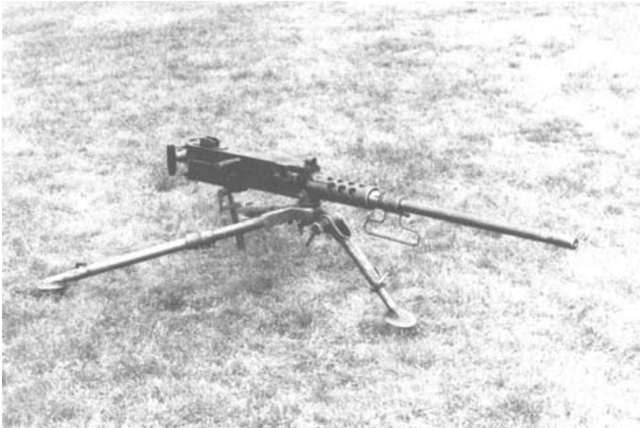
Figure 4-1. M2 .50 Cal on Tripod Mount, M3.
