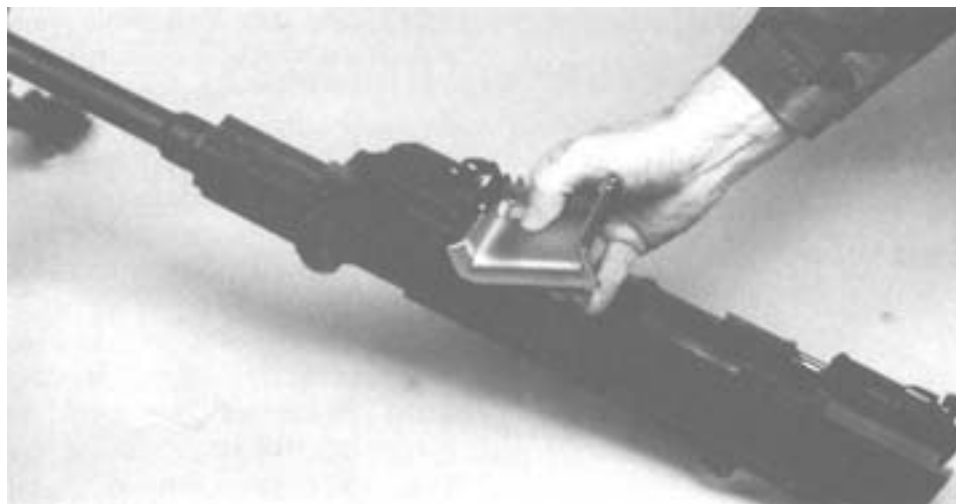
Figure 3-21. Aligning the Feed Tray Guides.
