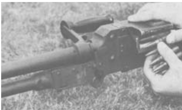
Figure 3-59. Loading, Cover Closed.
