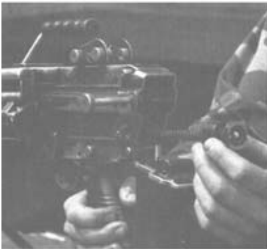
Step 2. Removing the Operating Rod.
