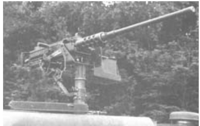
Figure 4-71. HMMWV Mount With MK64 MOD 5 Cradle.
