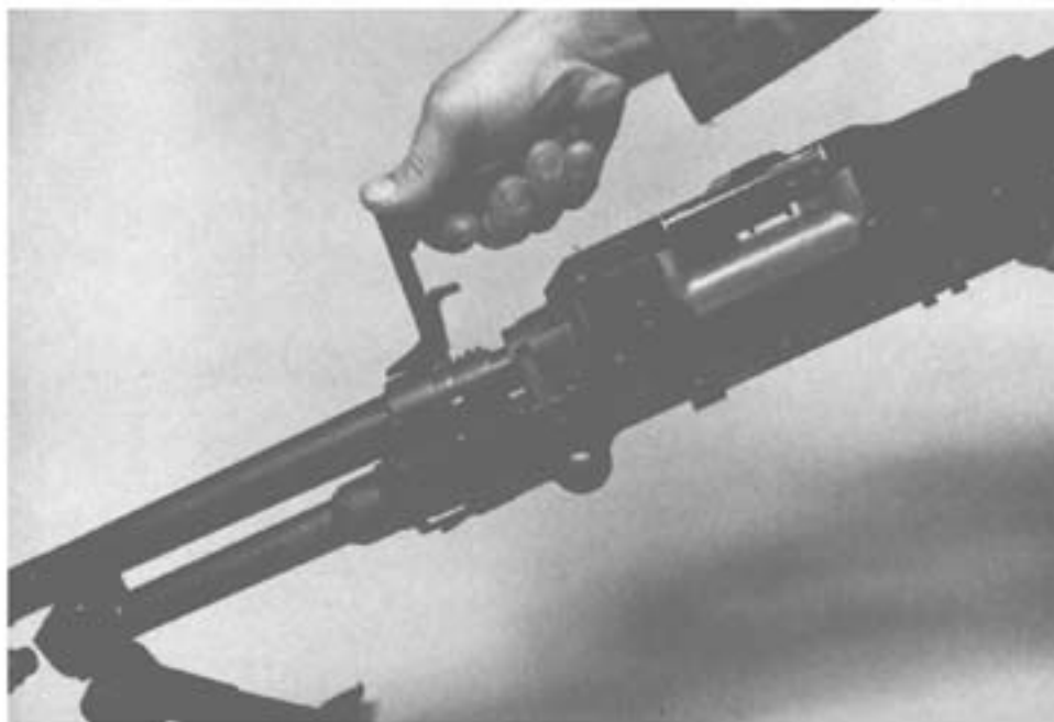
Step 2. Rotating Barrel Changing Handle Upright and Pulling Forward to Remove Barrel from Receiver.
