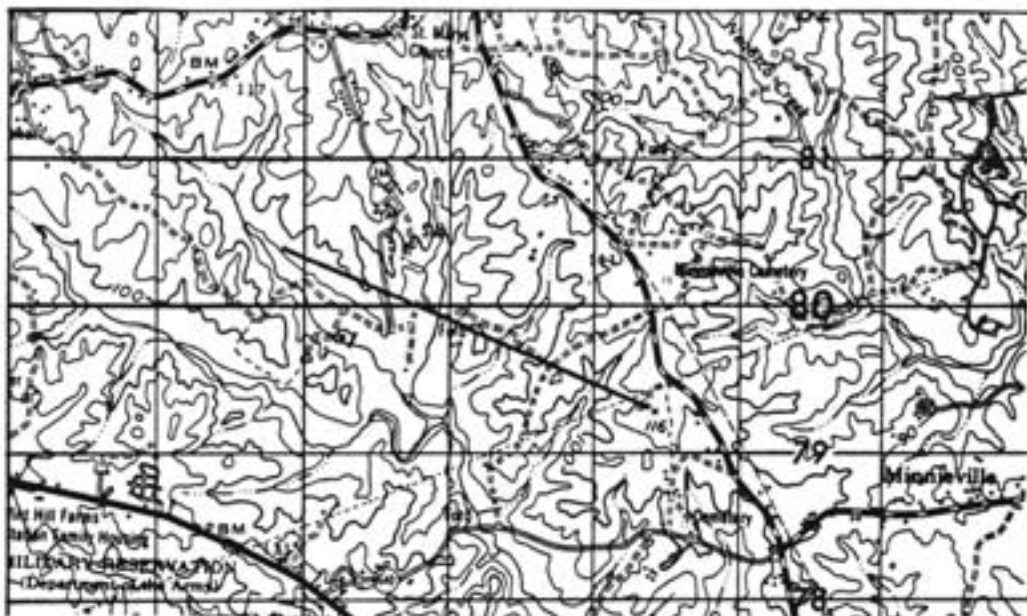
Figure 6-46. Profile Line (Map Contour Interval is 10 Feet).
