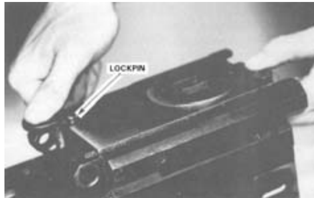
Figure 5-12. Lifting the Locking Pin.
