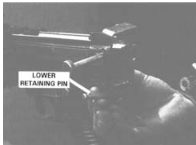
Figure 2-8. Removing the Buttstock and Buffer Group.
