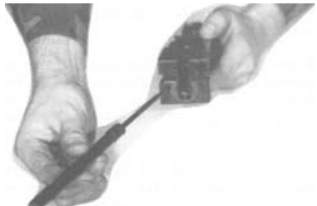
Figure 4-30. Removing the Firing Pin Extension Assembly and Firing Pin.
