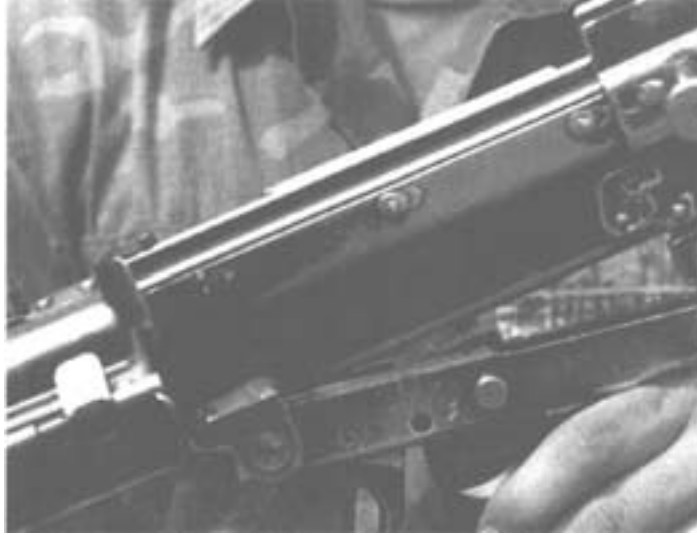
Figure 2-9. Removing the Trigger Group
