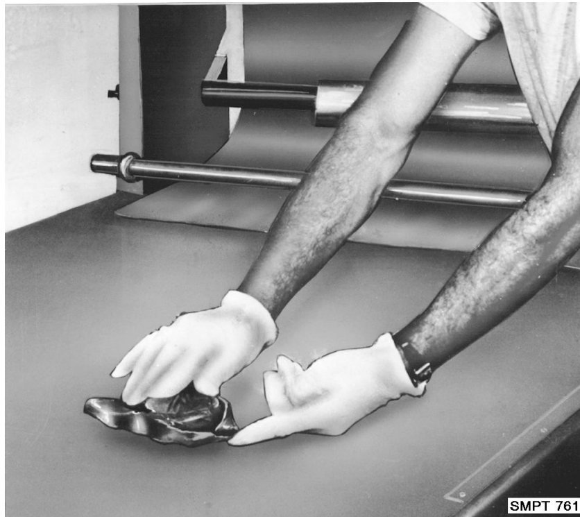
Figure 4-25. Method 20 - conform wrap to shape of item.
