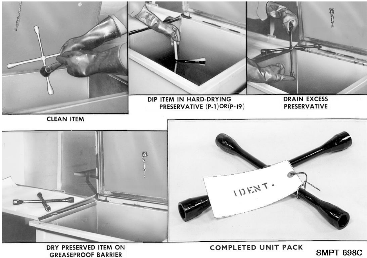
Figure 4-23. Application of Method 20 using a hard-drying preservative.
