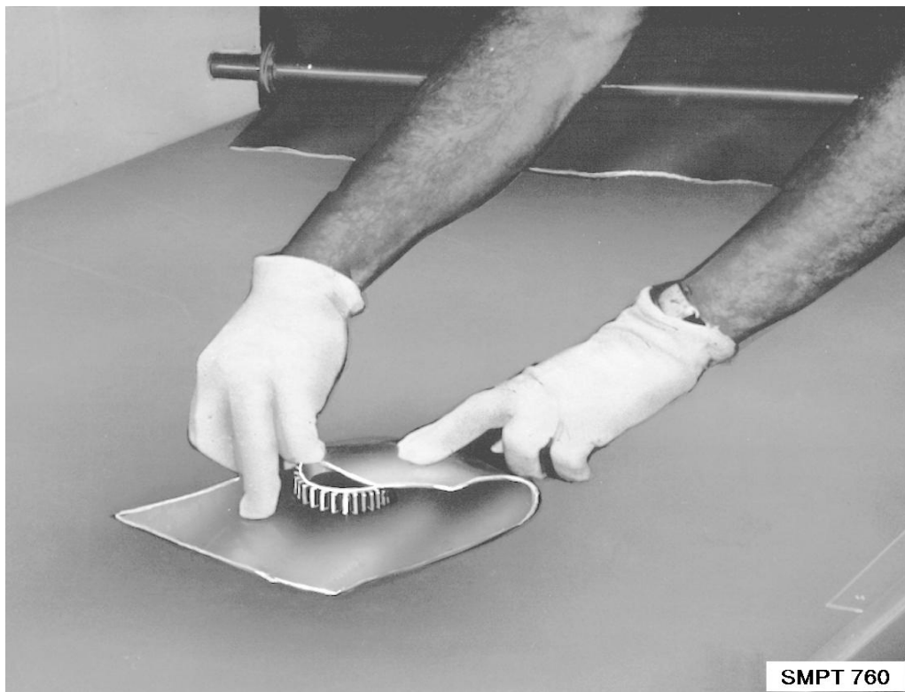
Figure 4-24. Method 20 - use large enough wrap to cover item completely.
