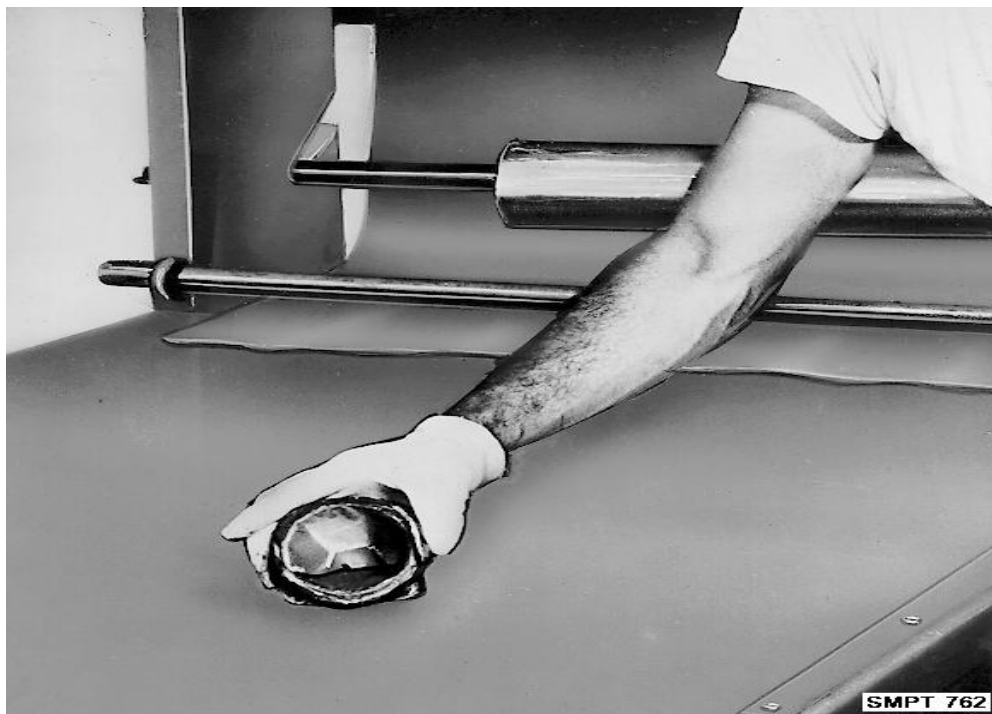
Figure 4-25. Method 20 - conform wrap to shape of item.
