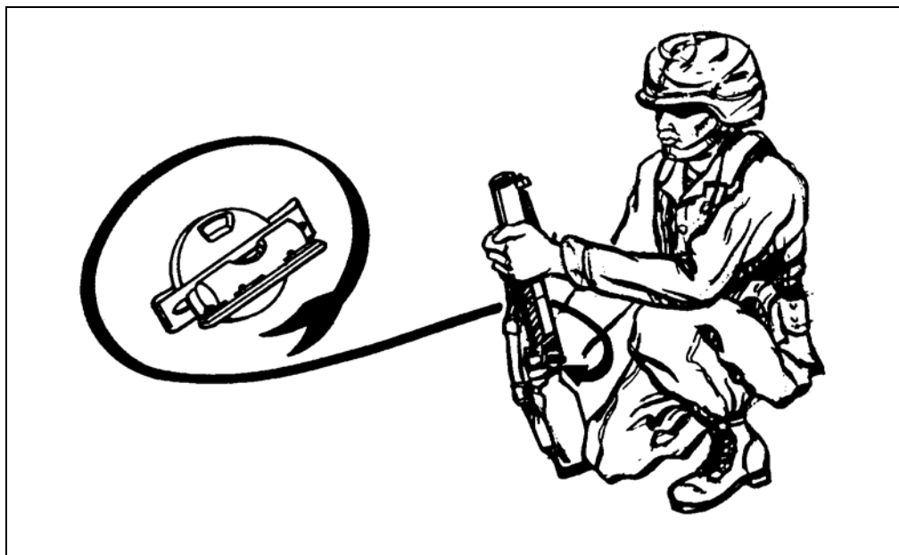
Figure A-23. Using the M5 rifle grenade sight.
