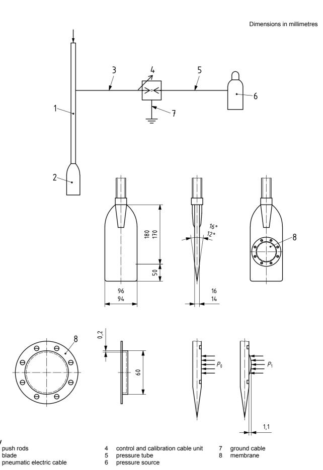
Figure 1 — Dilatometer equipment and definition of calculated in situ soil pressure (all measures in mm)
