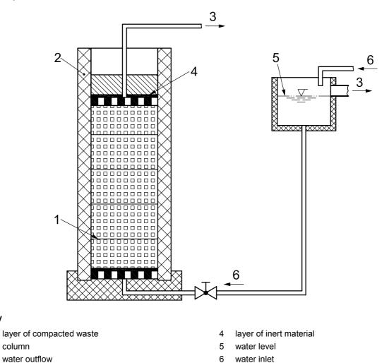
Figure A.1 — Saturation of the column by initial hydrostatic pressure
