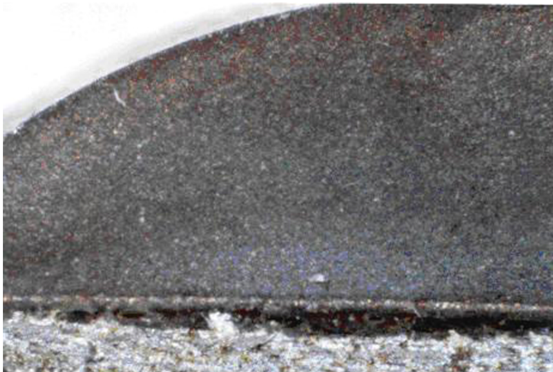
Figure 16 — Stable crack growth chain Type T, ald = 0,22 — Marked by heat tinting
