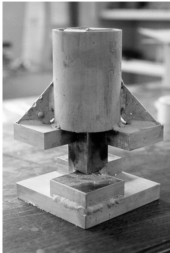
Figure 13 — Guided supporting and loading device for shear test ( continued )
