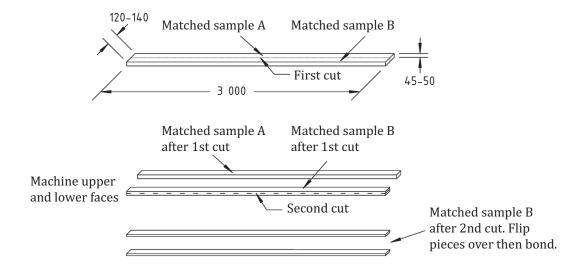
Figure 1 — Matched samples showing the cutting and bonding sequence.
