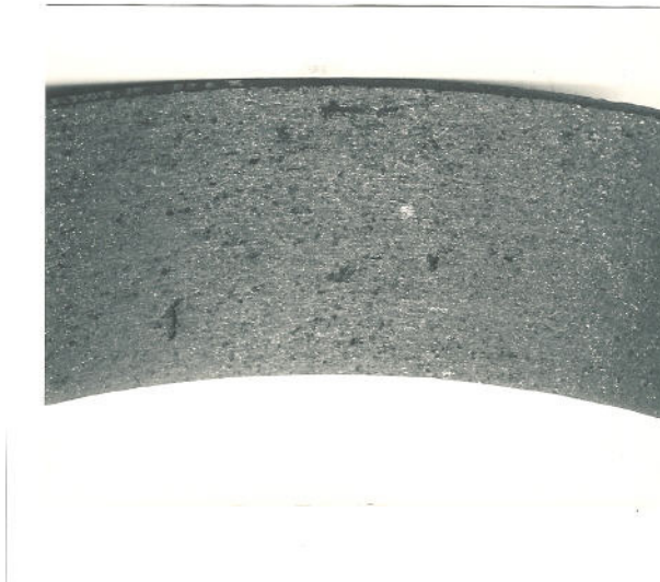
Figure 42 — Inside surface indentations
