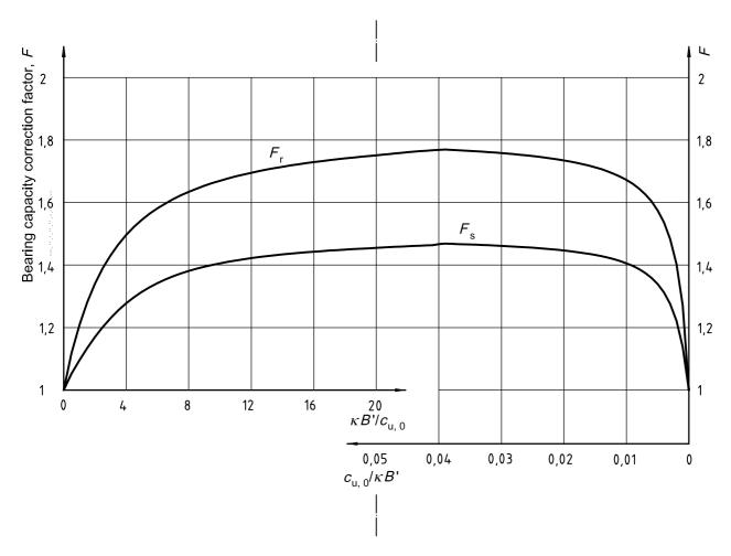
NOTE  $F_s$ , is for no friction at soil–foundation interface ("smooth" foundation),  $F_r$ , for friction equal to the shear strength of soil at the interface ("rough" foundation).
