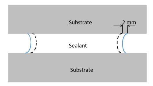
Figure 2 — 2 mm edge zone failure exclusion area
