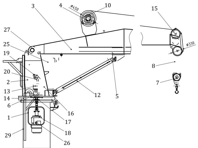
**A.1.2** A typical cylinder luffing deck crane is shown in Figure A.2.
