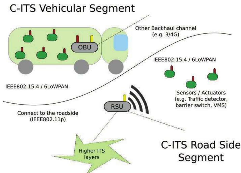
**Figure 3 — Example of 6LoWPAN nodes in ITS deployment**
