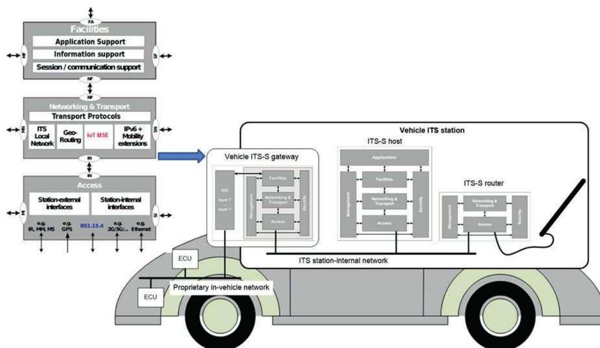
Figure 5 — Extended Vehicular ITS sub-system including 6LoWPAN
