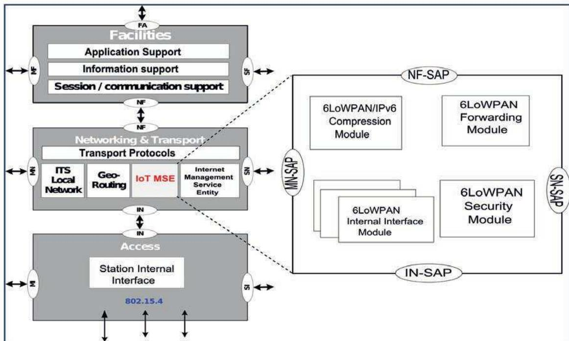
Figure 10 — ITS Station Unit: Modules implemented in BR (ITS-SCU) and Host (ITS-SCU)
