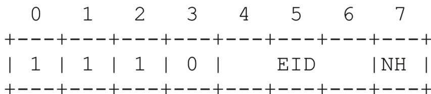
Figure 7 — LOWPAN NHC encoding for IPv6 Extension Header
