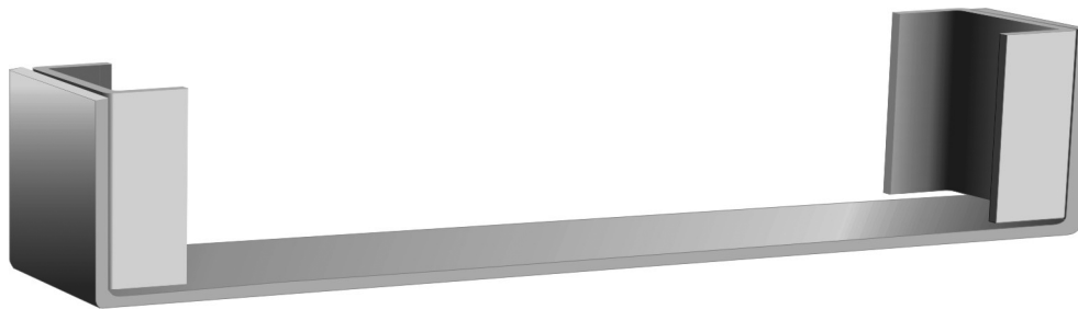
Figure 2 — Specimen jig to hold sandwiches
