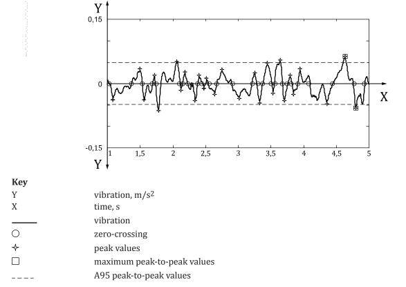
Figure 5 — Illustration of peak-to-peak calculations
