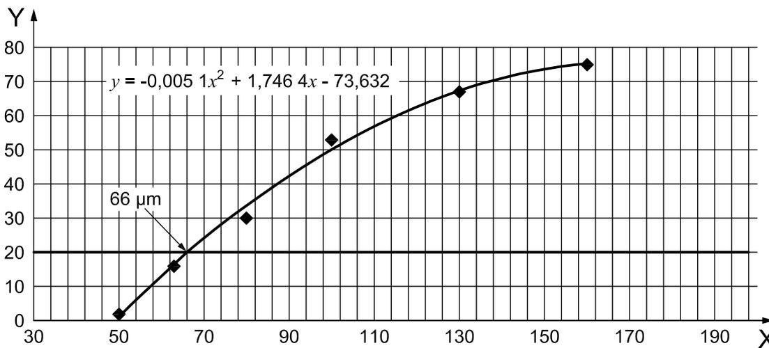
b) Interpolation of modulation depth vs. duplex wire diameter (corresponds to  $SR_b$ ). The 20 % value is determined from the intersection with the 20 % line resulting in  $iSR_b$  of 66  $\mu m$
