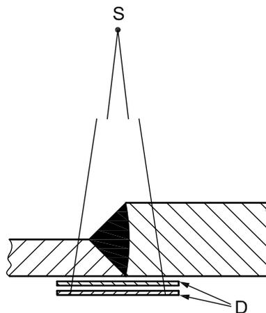
**Figure 19 — Multi-detector technique, applicable for CR**
