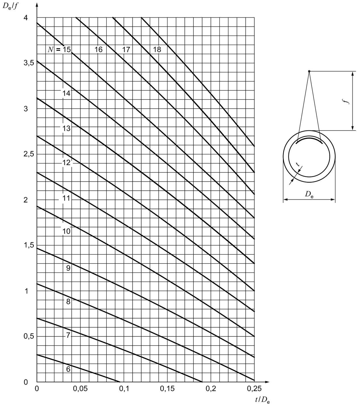
**Figure A.3 — Minimum number of exposures  $N$  for single wall penetration with source outside, with a maximum permissible increase in penetrated thickness  $\Delta t/t$  due to inclined penetration in the areas to be evaluated of 20 % (class A), as a function of ratios  $t/D_e$  and  $D_e/f$**
