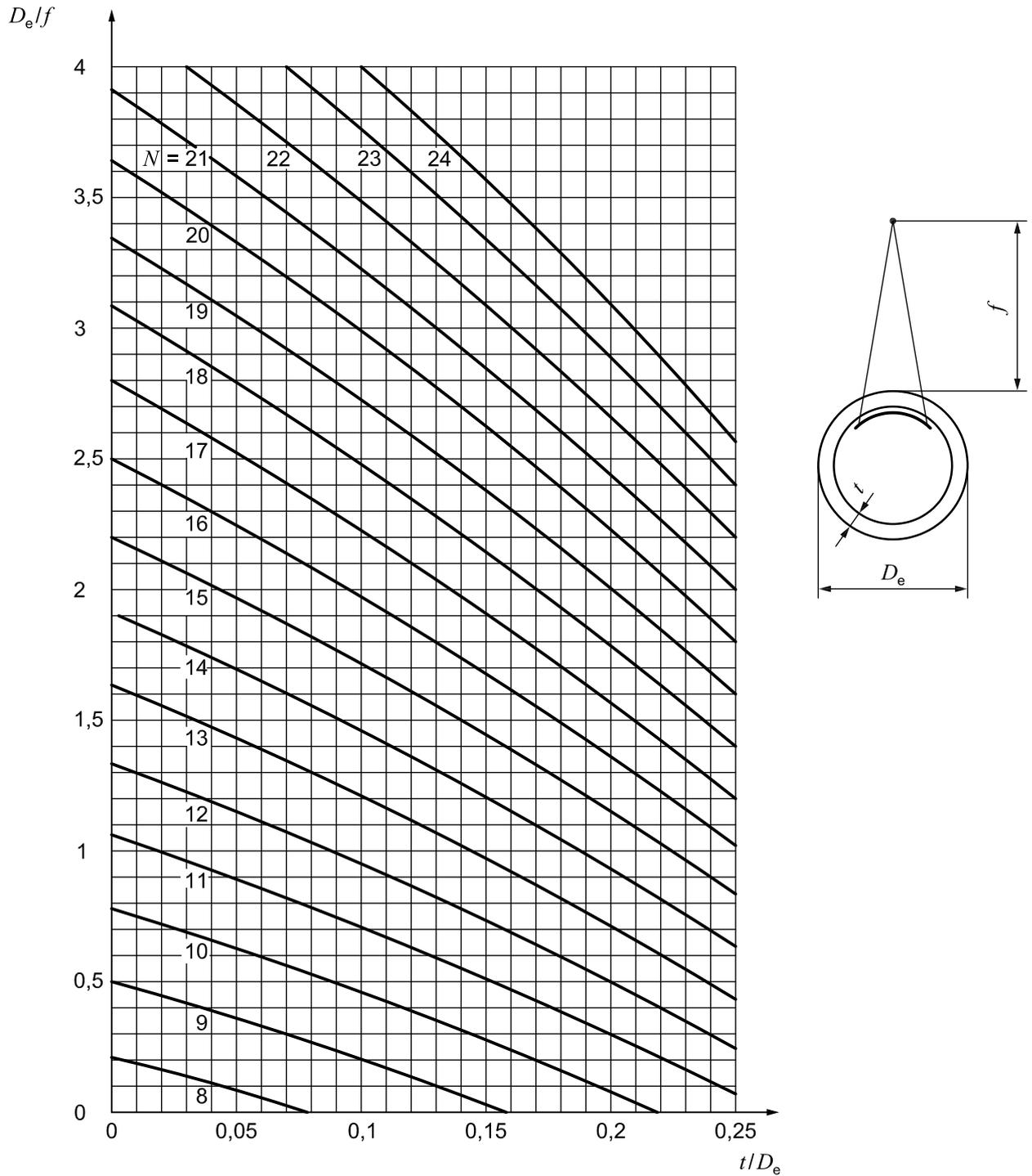
**Figure A.1 — Minimum number of exposures  $N$  for single wall penetration with source outside, with a maximum permissible increase in penetrated thickness  $\Delta t/t$  due to inclined penetration in the areas to be evaluated of 10 % (class B), as a function of ratios  $t/D_e$  and  $D_e/f$**
