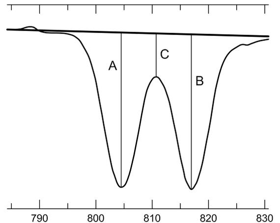
d) Scheme for calculation of the dip value (in %) with:  $dip = 100 \times (A + B - 2C)/(A+B)$
