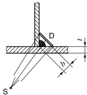
**Figure 18 — Test arrangement for penetration of fillet welds**
