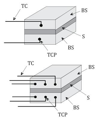
a) One-hole type Three-hole type b) TC thermocouple cartridge-type specimen TCP holes for temperature measurement
