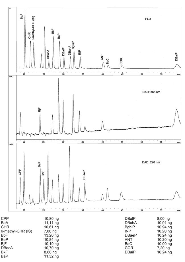
Figure B.1 — Chromatogram of a PAH calibration mixture
