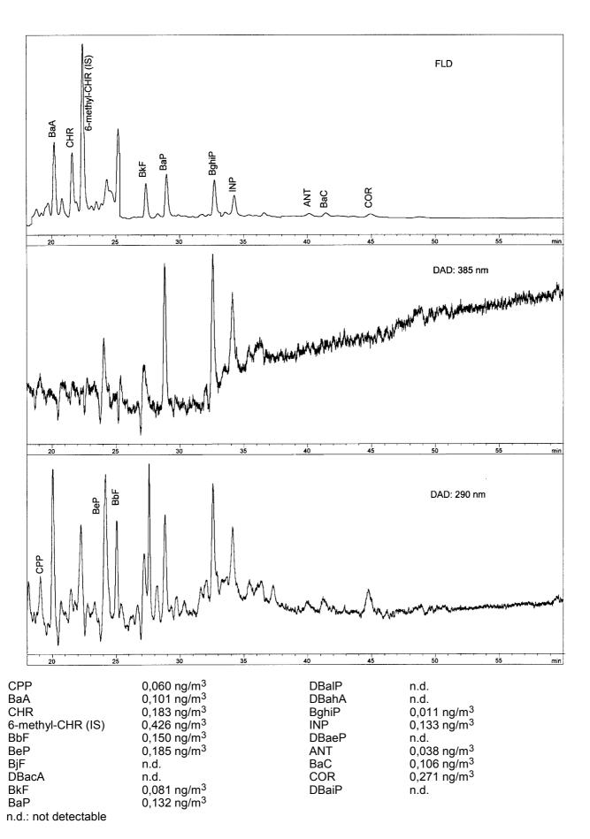
Figure B.2 — Chromatogram of an air sample
