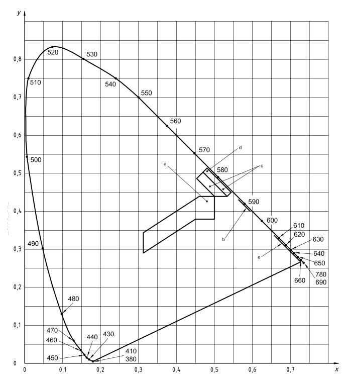
This diagram represents the zones of the CIE colour triangle, corresponding to the limits in Table B.1.
