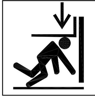
Figure A.17 — Example of pictorial using arrows to represent the direction of motion of machine components
