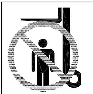
Figure C.5 — Do not stand under the forks
