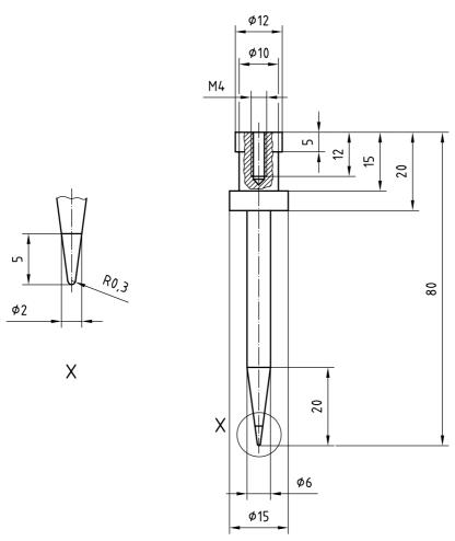
Figure I.1 — Reference spike, annealed
