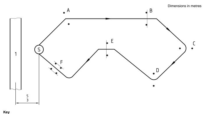
Figure C.1 — Test course for bridge or gantry cranes
