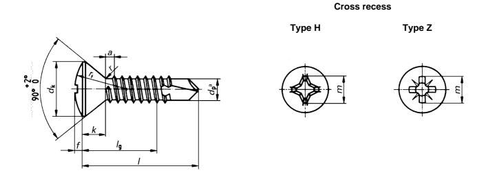
The function of the drilling point (diameter  $d_p$ ) is specified in ISO 10666.
