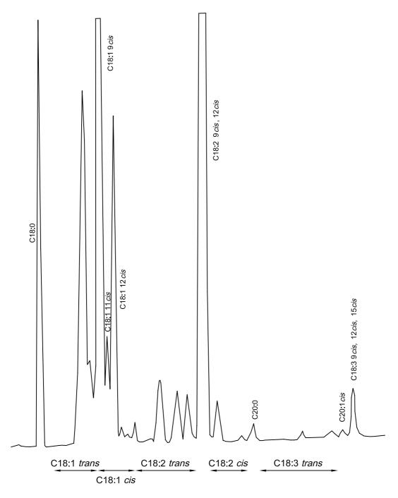
NOTE Obtained using a 60 m  $\times$  0,25 mm  $\times$  0,20  $\mu$ m SP-2340 column (Supelco) at 190 °C (isotherm). The *cis* and *trans* fatty acid isomer retention areas are indicated on the chromatogram.
