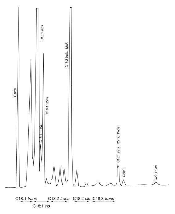
NOTE Obtained using a 50 m  $\times$  0,22 mm  $\times$  0,25  $\mu$ m BPX-70 column (SGE) at 198 °C (isotherm). The *cis* and *trans* fatty acid isomer retention areas are indicated on the chromatogram.
