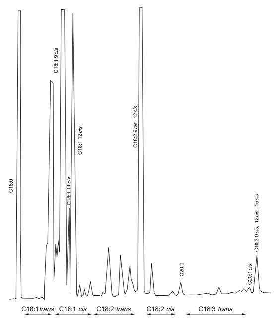
NOTE Obtained using a 50 m  $\times$  0,25 mm  $\times$  0,20  $\mu$ m CP<sup>TM</sup>-Sil 88 column (Chrompack) at 175 °C (isotherm). The *cis* and *trans* fatty acid isomer retention areas are indicated on the chromatogram.
