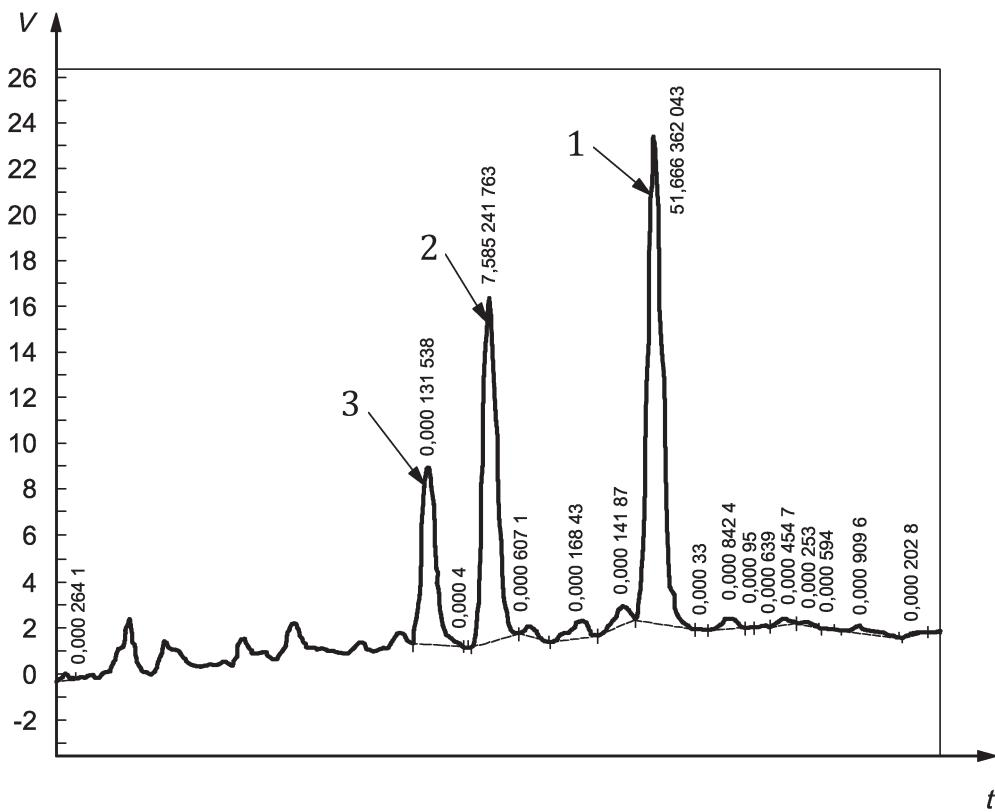
**Key** $V$  HPLC absorbance/mV $t$  time/min1 benzo[*b*]chrysene (internal standard)2 benzo[*a*]pyrene3 benzo[*k*]fluoranthene**Figure 1 — Typical chromatogram**
