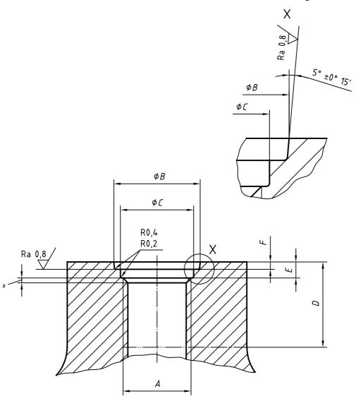
Chamfer 45 ° × root diameter.
