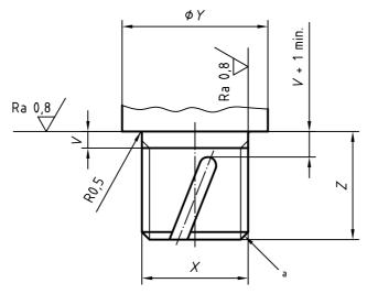
a Chamfer 45° × root diameter.
