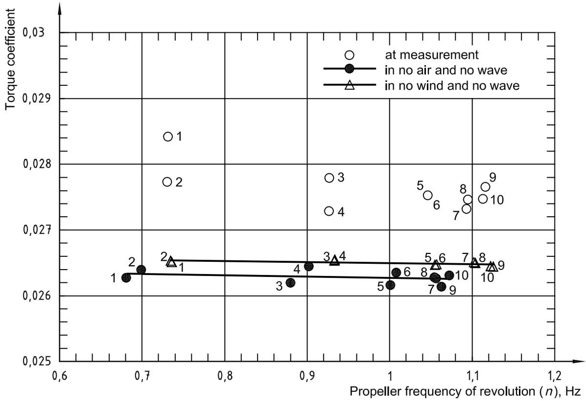
Figure 6 — Example of torque coefficient curves and propeller frequency of revolution
