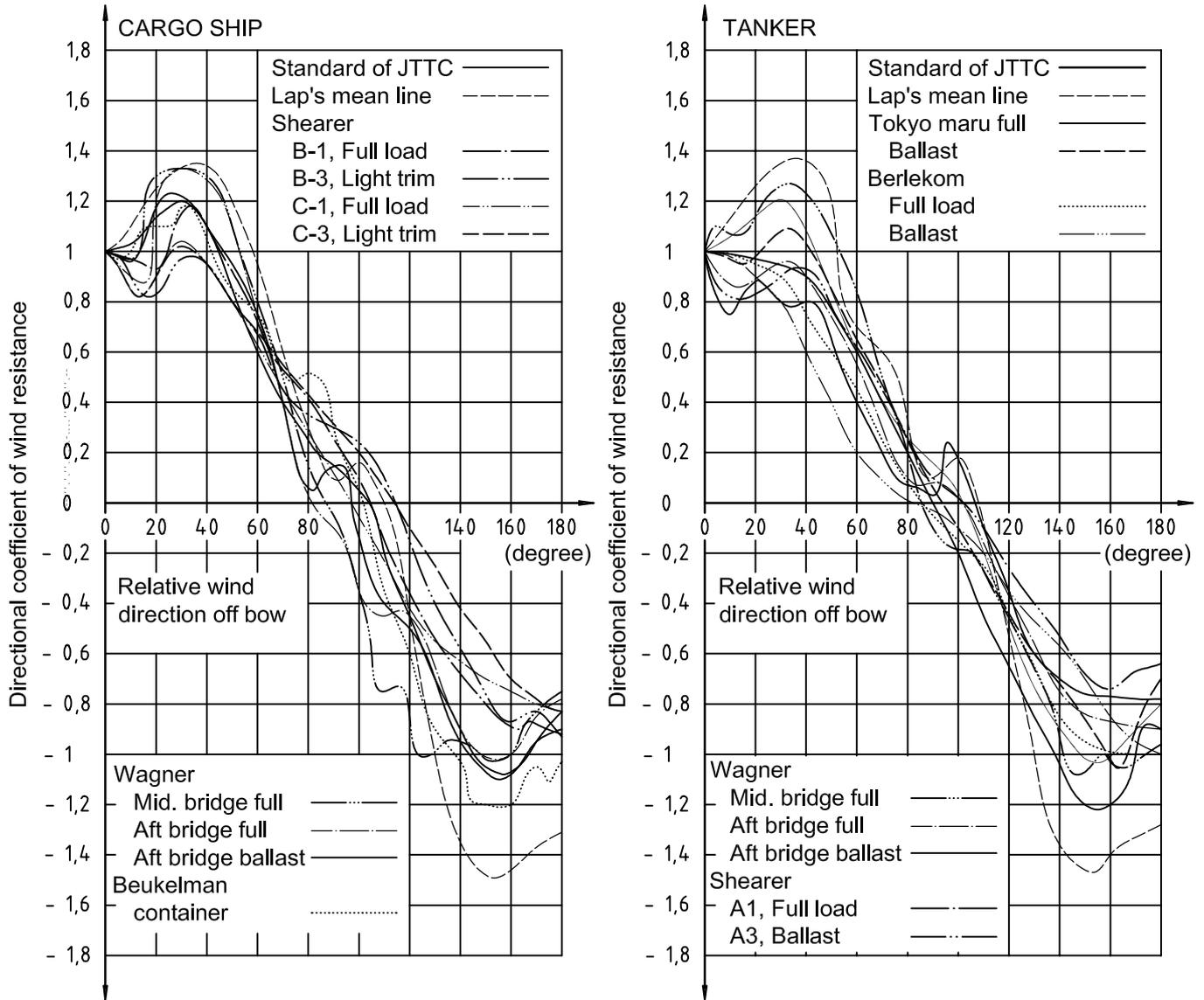
Figure A.2 — Directional coefficient of wind resistance
