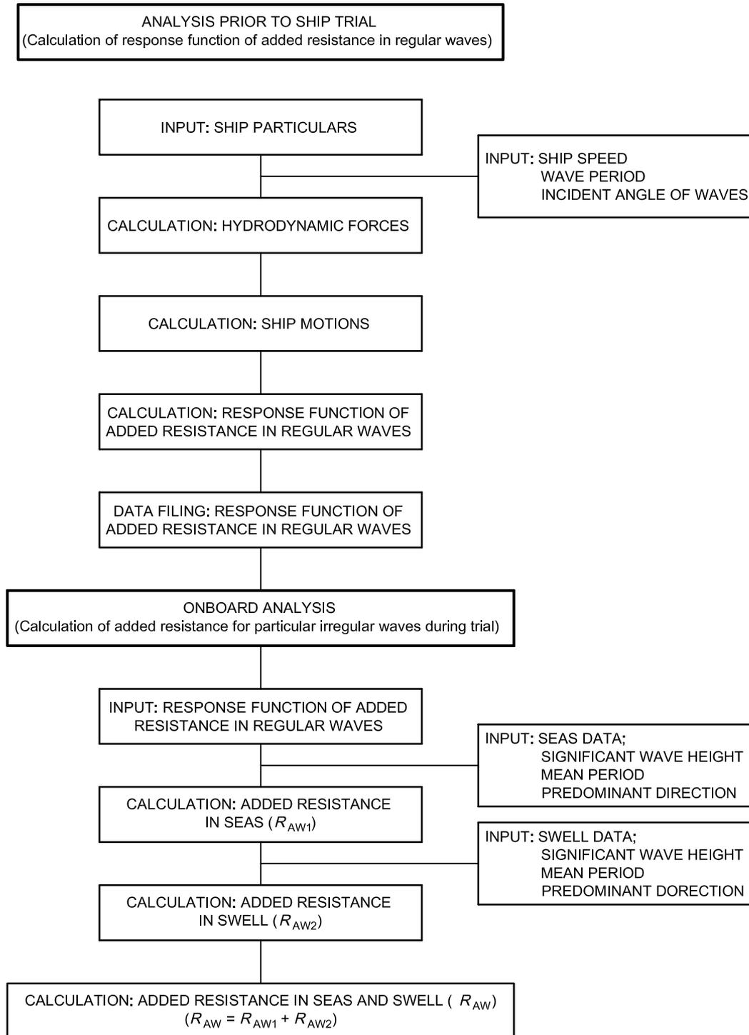
Figure B.1 — Flowchart for calculation of resistance increase in waves
