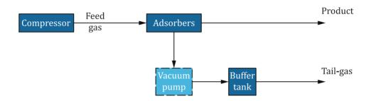
Figure 1 — Example of typical equipment in PSA system for hydrogen separation and purification
