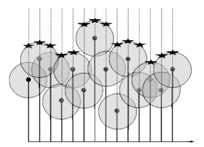
NOTE The centre of the disk is positioned at every input data point. The stars are the maximum height of all the results calculated by adding the coordinates of input points (filled dots) to the coordinates of sampled points on the circle.
