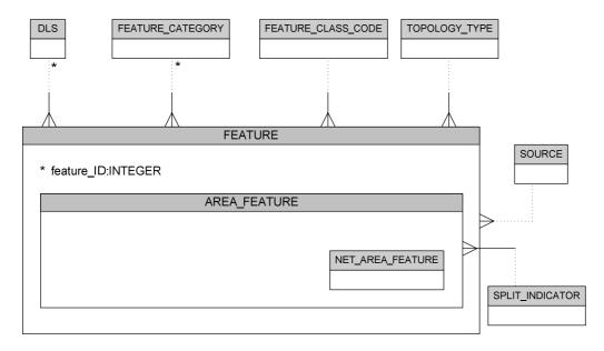
For Non-Explicit Topology Area Features, topology is not expressed with topological primitives, but instead can be derived from its NET Polygon geometry.
