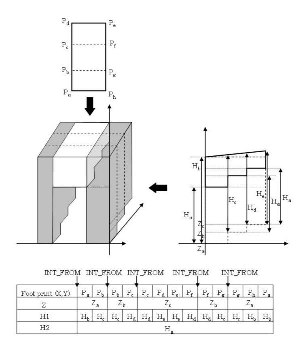
Figure 226 — Example for 231\* coordinate mask
