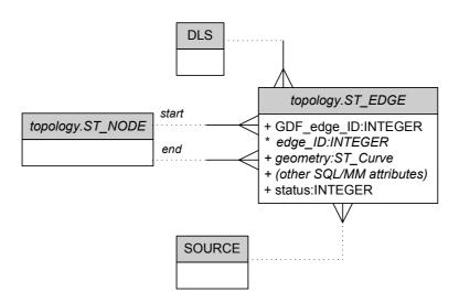
Using elements of ISO 13249-3, individual Edges are represented by SQL/MM ST Edge. SQL/MM provides edge ID, geometry, and additional SQL/MM specific attributes. Edge ID is unique within a TopoGeo "topology", equivalent to a planar graph. Here "topology" is the name of the SQL schema which owns the ST Nodes,
