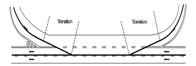
Figure 143 - Schematic example of road centreline transition at an entry/exit lane
