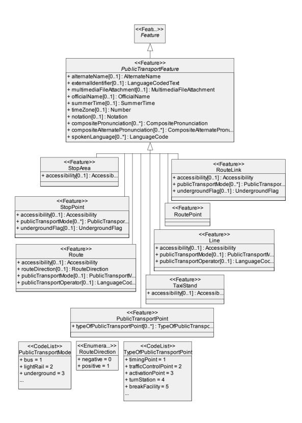
Figure 122 — The Conceptual Data Model for Attributes of Public Transport Features
