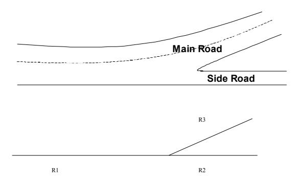
Figure 184— Example of a Through Route
