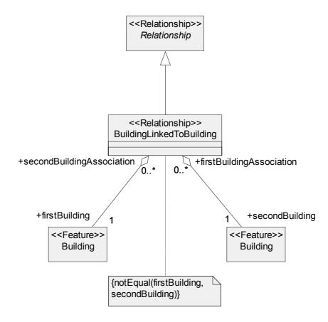
Figure 171 —The Conceptual Data Model for the Building Linked To Building Relationship
