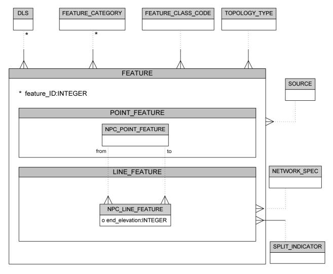
Non-planar connectivity Topology Type of Line Features can have a from and a to non-planar connectivity topology type Point Feature.
