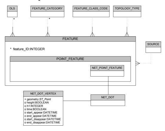
For Non-Explicit Topology Point Features, topology is not expressed by a topological primitive, but instead can be derived from its NET Dot geometry.
