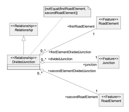
Figure 147 — The Conceptual Data Model for the Divided Junction Relationships
