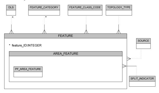
GDF extends *ST\_Face* with a GDF-specific GDF Face ID, unique within a Section. They have a mandatory Boolean extended area geometry information flag and optional geometrical type, slope, aspect, and light (shading) value attributes. They can also include an integer source ID referencing Source (see 14.4.3.8).
