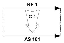
The source Line Feature, Road Element RE1, is assigned to the single, entire target Line Feature, Anchor Section AS101, representing source feature number 1, with a single Correspondence C1 having a Correspondence Order of 1 (one) and a Validity Direction Attribute equal to "same direction".
