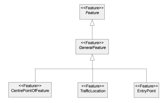
Figure 92 — The Conceptual Data Model for General Features
