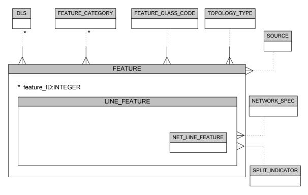
For Non-Explicit Topology Line Features, topology is not expressed with topological primitives, but instead can be derived from its NET Polyline geometry.
