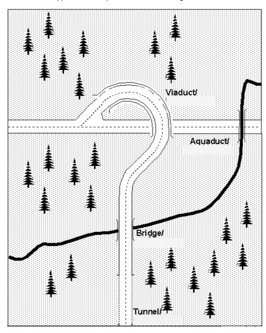
Figure 140 — Examples of different Structure Types
