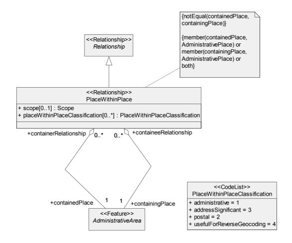
Figure 160 — The Conceptual Data Model for the Place within Place Relationship
