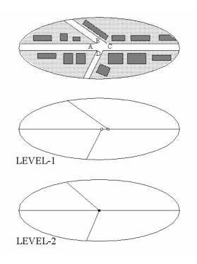
Figure F.5 — A four-valent crossing with two Junctions and one Intersection
