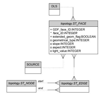
Each planar full Topology Type of Area Feature can have a single topological representation. Using elements of ISO 13249-3, the topological representation is by a set of SQL/MM defined faces (ST\_FACE). Faces do not have their own geometry values but the geometry can be constructed from the geometry of their contributing
