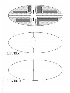
Figure F.12 — An example of Level-2 formation of Intersections at crossings with traffic islands
