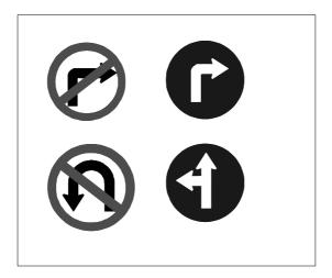
Figure 180 — Traffic Signs for Prohibited Manoeuvre and Restricted Manoeuvre
