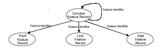
Figure 218 — Pointer relations among features in the non-explicit topology model (the reverse direction for each pointer relation is not shown)
