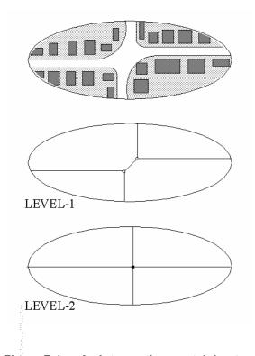
Figure F.4 — An Intersection containing two **Junctions**
