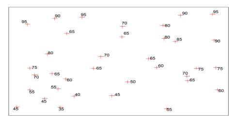
Figure 78 – Example of reduced TIN representation in terms of TIN Nodes
