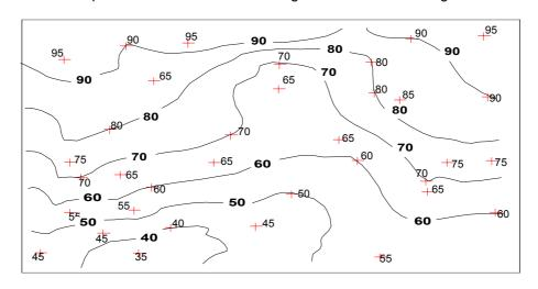
Figure 79 – Example of contour line representation
