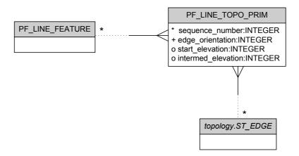
Each Planar Full Topology Type of Line Feature may have a single topological representation. Using elements of ISO 13249-3, the topological representation is by a list of *SQL/MM defined edges (ST\_Edge)*, ordered by sequence number. The Edge orientation indicates whether the Line Feature uses each Edge in the direction it is defined, as dictated by the start and end Nodes.
