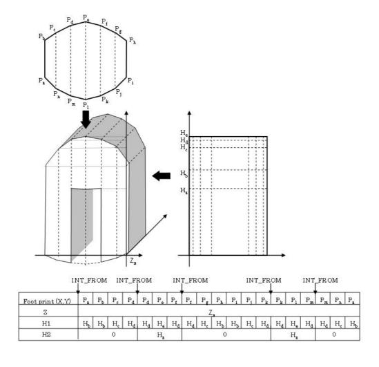
Figure 224 — Example for 132\* coordinate mask
