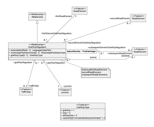
Figure 161 — The Conceptual Data Model for the Give Way Regulation Relationship
