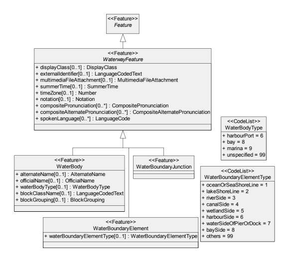
Figure 117 — The Conceptual Data Model for Attributes of Waterways
