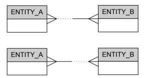
When appearing on an ERD, this should always be questioned. It is usually the case that there is additional information about the relationship itself (not about either of the entities individually). If this is the case, the appropriate solution is to add an additional (intersect) entity which will eliminate the many-to-many associations and will be a place where the relationship attributes can go.
