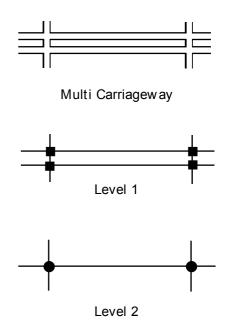
Figure F.6 — A six-valent crossing with six Junctions and one Intersection
