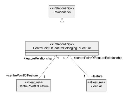
Figure 159 — The Conceptual Data Model for the Centre Point of Feature belonging to Feature Relationship
