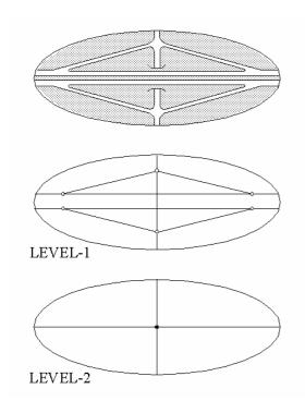
Figure F.16 — An example of a level-2 representation of an Interchange
