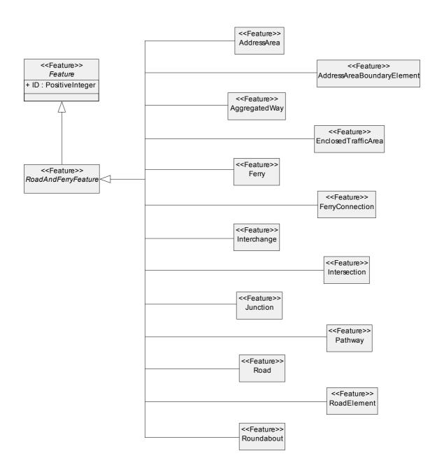
Figure 27 — The Conceptual Data Model for Roads and Ferries
