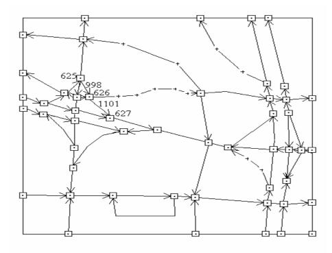
Figure 190 — Example of topological Level-0 representation of Roads and Ferries, Administrative Areas and Waterways in planar or non-planar topology
