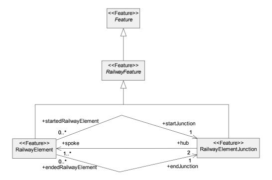
Figure 82 — The Conceptual Data Model for Railways
