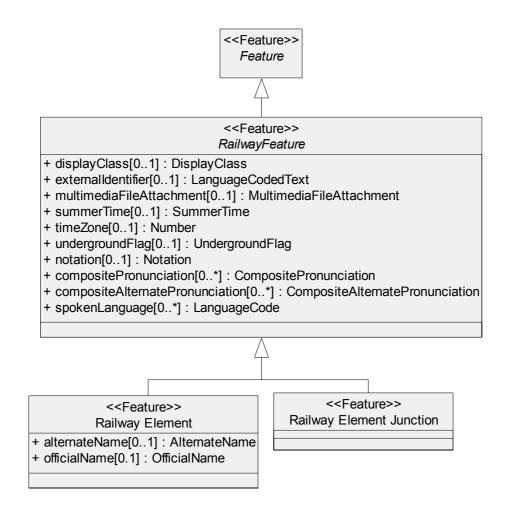
Figure 116 — The Conceptual Data Model for Attributes of Railway Features
