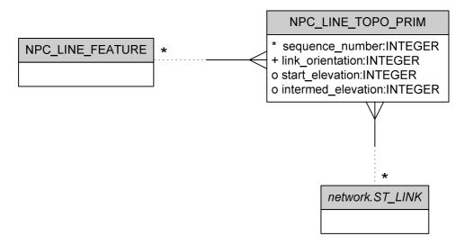
Each non-planar connectivity Topology Type of Line Feature may have a single topological representation. Using elements of ISO 13249-3, the topological representation is by a list of *SQL/MM defined links (ST\_Link)*, ordered by sequence number. The link orientation indicates whether the Line Feature uses each Link in the direction it is defined, as dictated by its start and end Nodes.
