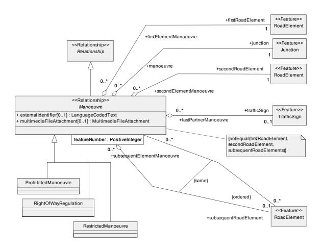
Figure 146 — The Conceptual Data Model for Manoeuvre Relationships
