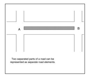
Figure 44 — Road Elements as separated Carriageways
