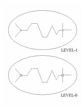
Figure 192 — Representation of a segmented line
