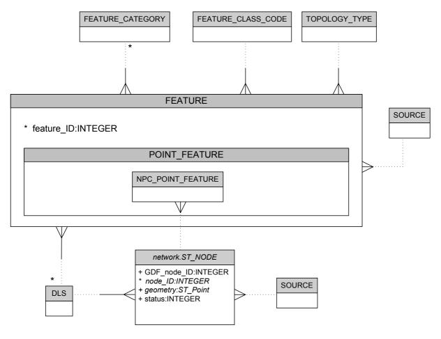
If the Point Feature has a Node, then both must be in the same Section (have the same DLS). They may have different Sources.
