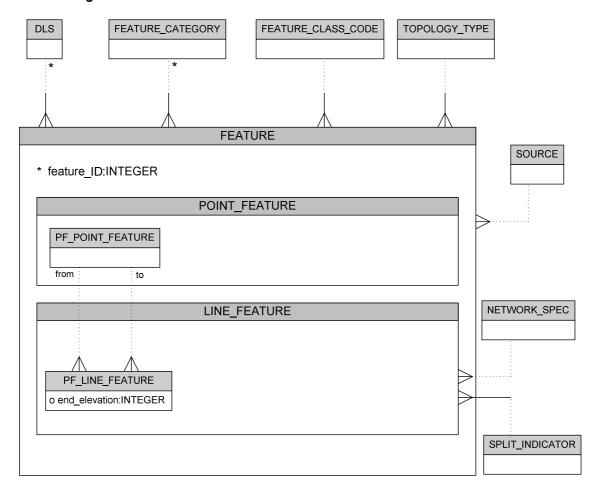
Planar full topology type of Line Features can have a from and a to planar full topology type Point Feature.
