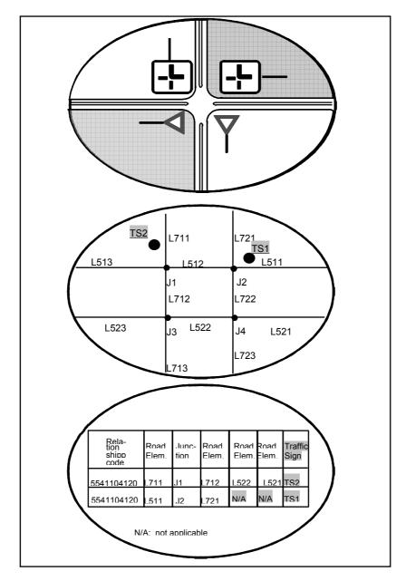
Figure 179 — Example of Right of Way Regulation
