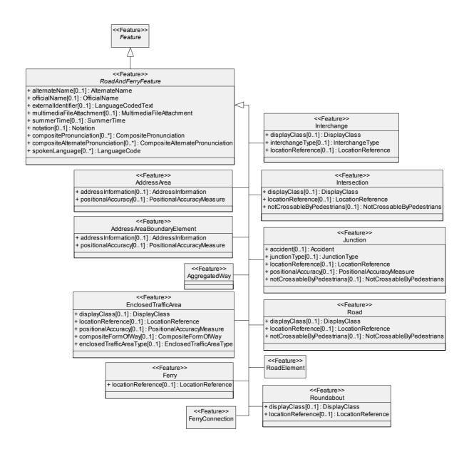
Figure 100 — The Conceptual Data Model for Attributes of Roads and Ferries
