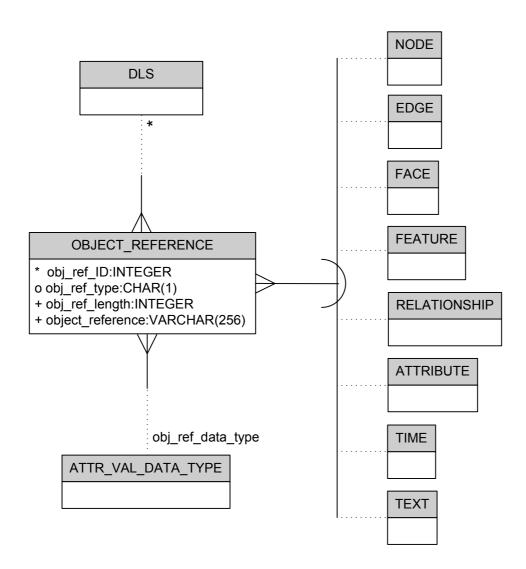
Object References refer to a single object (Feature, Relationship, Node, Edge, Face, Time, Text, or Attribute). They are uniquely identified by an object reference ID, unique within a DLS. The DLS of the object reference is the same as the DLS of the object.
