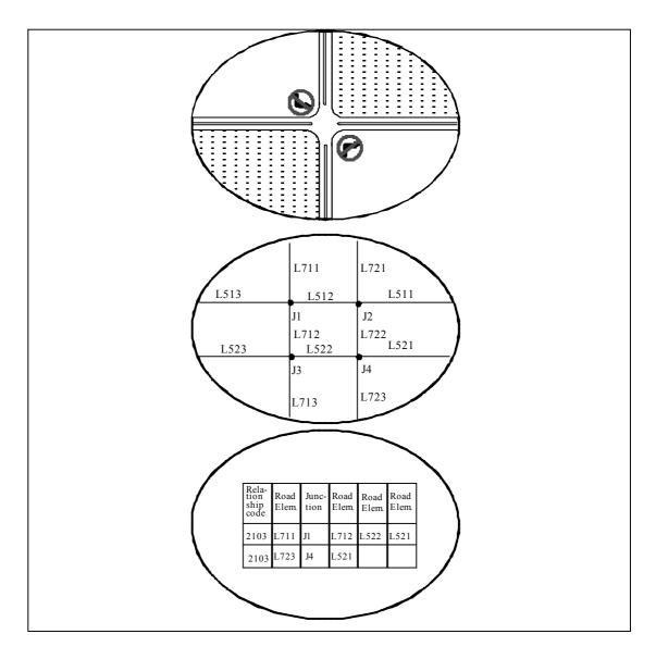
Figure 182 — Representation of a Prohibited Manoeuvre
