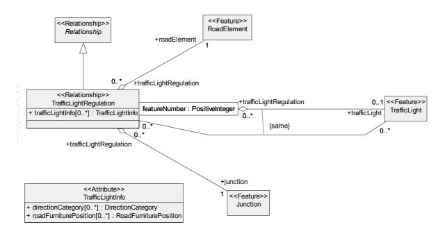
Figure 166 — The Conceptual Data Model for the Traffic Light Regulation Relationship
