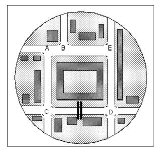
Road Element CD is independent of other Road Elements. When CD is blocked, traffic can still flow on other elements.
