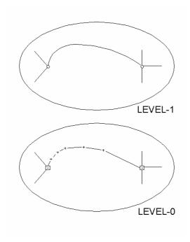
Figure 193 — Representation of curved linear objects
