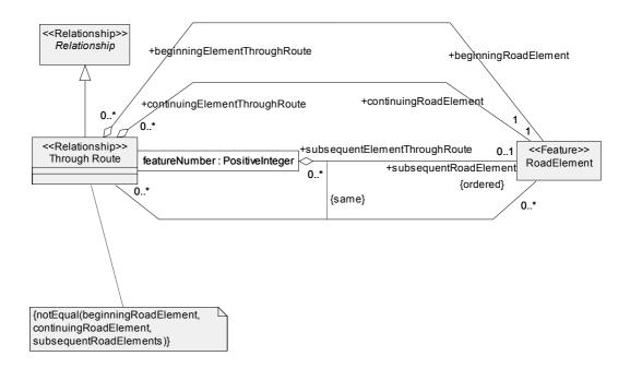
Figure 148 — The Conceptual Data Model for the Through Route Relationship
