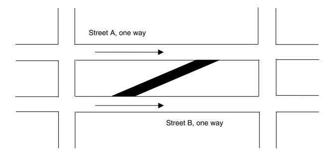
Figure 138 — Example of a Slip Road of type "Other"
