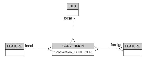
In this Logical Model, the DLS of the Conversion entity is shown because it's unique identifier is needed to make the conversion ID unique in the database. Because this DLS is the same as the DLS that is part of the unique identifier for the local Feature, it does not have to appear twice in the physical implementation.
