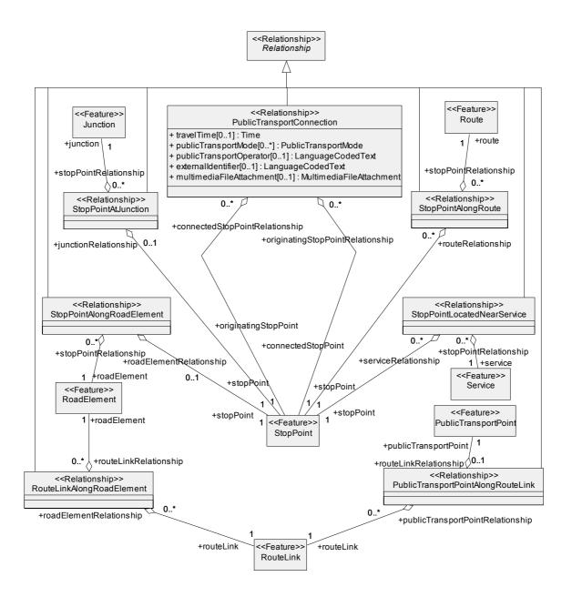
Figure 158 — The Conceptual Data Model for the Relationship involving Public Transport Features
