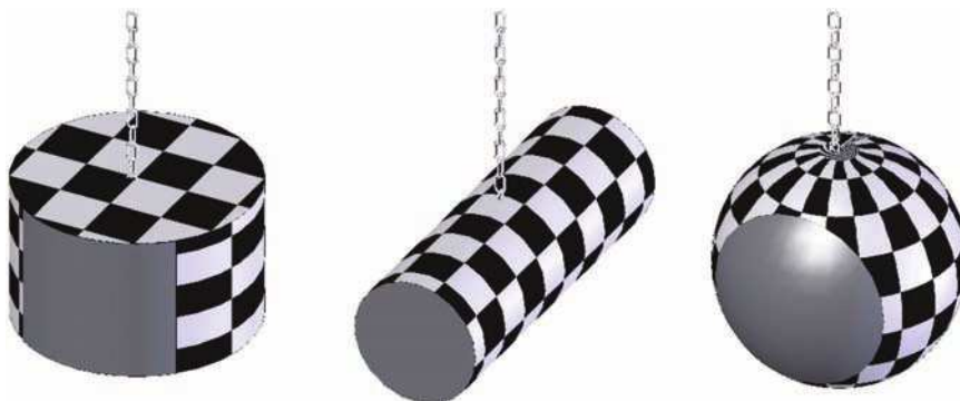
Figure C.2 — Sample of hard bodies showing impact area
